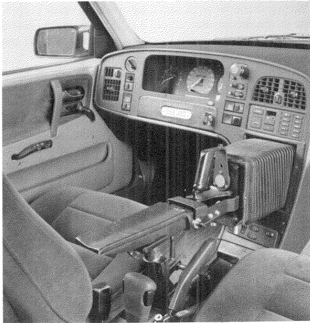
Figure 1. Steer-by Wire and a Joy-stick Installed in a Saab 9000
