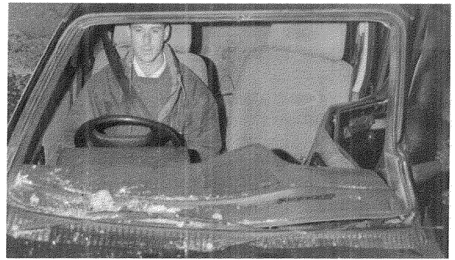
Figure 1. Front, Interior View of a Vehicle With Side Impact Damage, an Occupant is Seated on the Non-Struck Side
