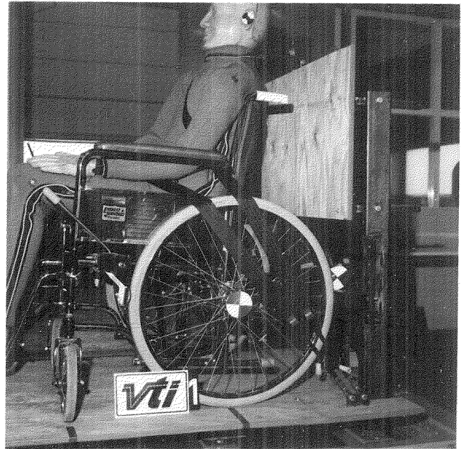
Figure 5. The Restraint System Used in the Impact Tests
