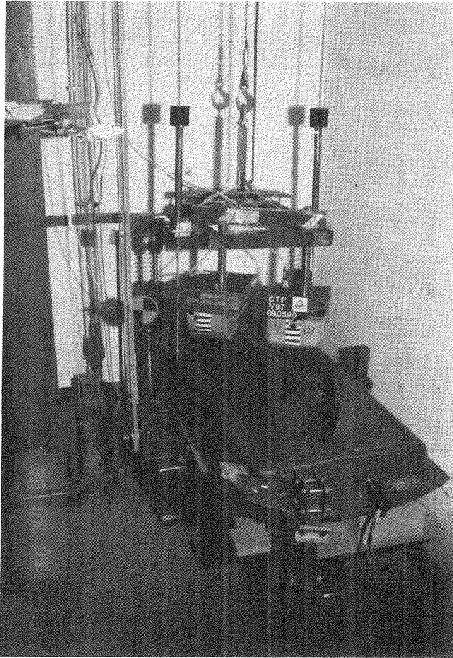
Figure 3. Dynamic Impact Test Rig with a Production Volvo 480 Door Assembly
